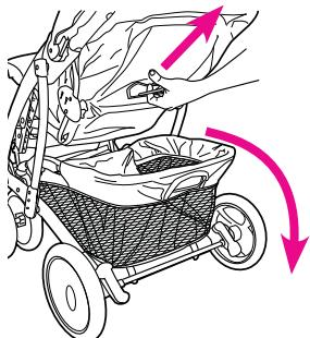
**To recline:** lift up back of canopy, and squeeze recline wire on back of seat.
